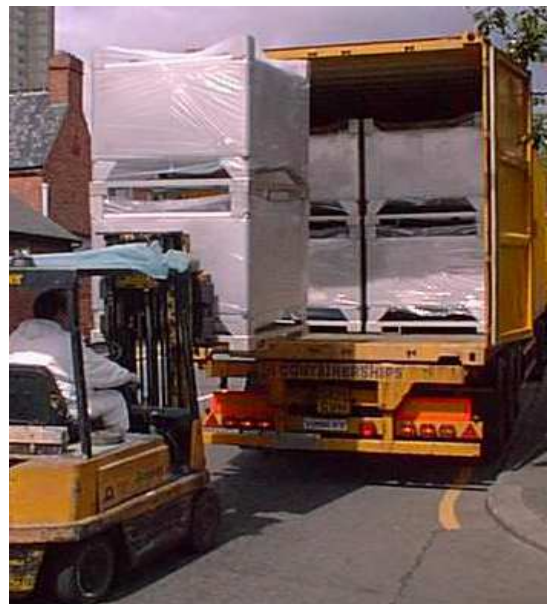
Stacked 2 high, 20 MC cubes can fit into a 20 ft ISO container, ie. 20,000 Litres of product
